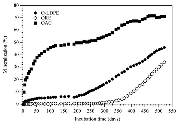
Fig. 7. Mineralization profiles of Q-LDPE, residue to solvent extraction (QRE), and acetone extract (QAC) of Q-LDPE sample in soil burial test.
