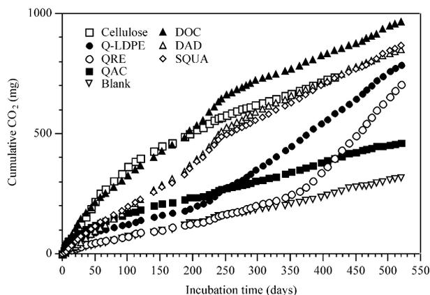
Fig. 6. Cumulative  $\text{CO}_2$  emissions of Q-LDPE, residue to solvent extraction (QRE), acetone extract (QAC) of Q-LDPE sample, and reference aliphatic hydrocarbons (Docosane DOC,  $\alpha,\omega$ -docosandioic acid DAD, and squalane SQUA) in soil burial test.
