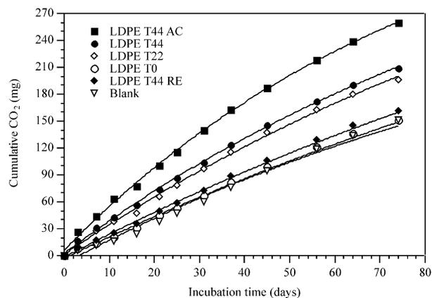
Fig. 13. Cumulative CO<sub>2</sub> emissions of acetone extract of the LDPE specimen submitted to 44 days oxidative thermal treatment (LDPE T44 AC), entire LDPE film specimens collected after 22 (LDPE T22) and 44 (LDPE T44) days thermal treatment, residues to extraction (LDPE T44 RE), original LDPE film (LDPE T0) and blank in a soil burial test.
